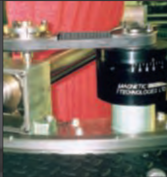
Torque limiting application using Model 610 with custom adaptor and gear.
