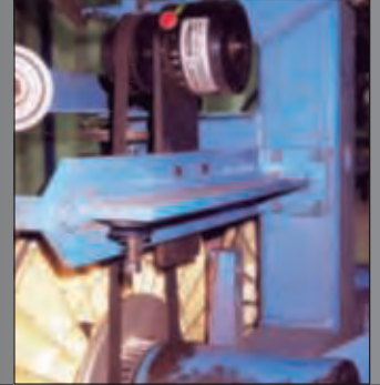
Retrofit application using Model 523 and 700-002M Mounting Bracket on Twister.
