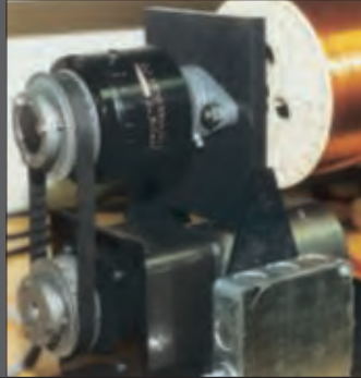
Powered take-up: Two flanged bearings support shaft and the housing is powered.
